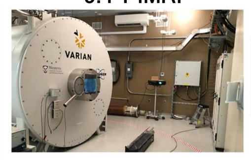
Gradient strength: 1.5 mT/m/A Coil: 8-channel receive coil
